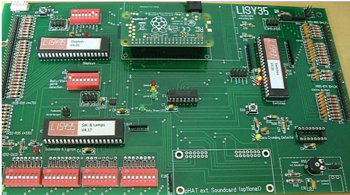
Picture 3: LISY35 after Step 4. 'Ready to go'(HW Version 1.3)
