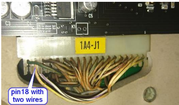
Picture 4: display connector with two wires at pin18
