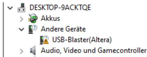
**You also need to install the driver for your USB Blaster.** The driver comes together with the installation of the programmer and is located in the 'driver' subdirectory.
