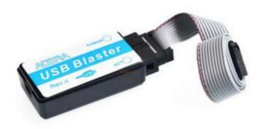
2) Start the programmer, make sure in the Hardware setup ,USB-Blaster' is visible and set the Mode to ,Activeserial Programming'
