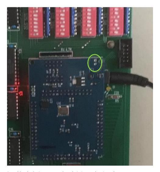
Do solder the 2-pin connector here (missing on the picture)
