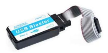
2) Start the programmer, make sure in the Hardware setup ,USB-Blaster' is visible and set the Mode to ,JTAG'
